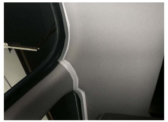
Keep tucking after the B-pillar along the headliner, and continue tucking down the C-pillar until you get to the black plastic trim. Again pull at it slightly and tuck the wires in. Then push them into the space between the fixed seat back and the C-pillar. If you reach around the left side of the fixed seatback (with the folding seatback folded down) you meet your hands in there somewhere to pull the wires the rest of the way through.
