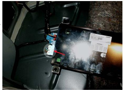
We are interested in the red wire with black stripe. This is constant 12v. (Note, the connector on the left in this picture is for the speakers, you do not need to remove it)
