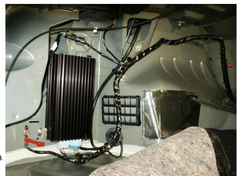
Here is the amp removed, the power connector is highlighted. Use a screw driver to push the tab in, and the connector slides right out.
