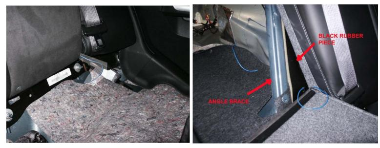
Run the wire along the sidewall of the trunk, tape it in place.
