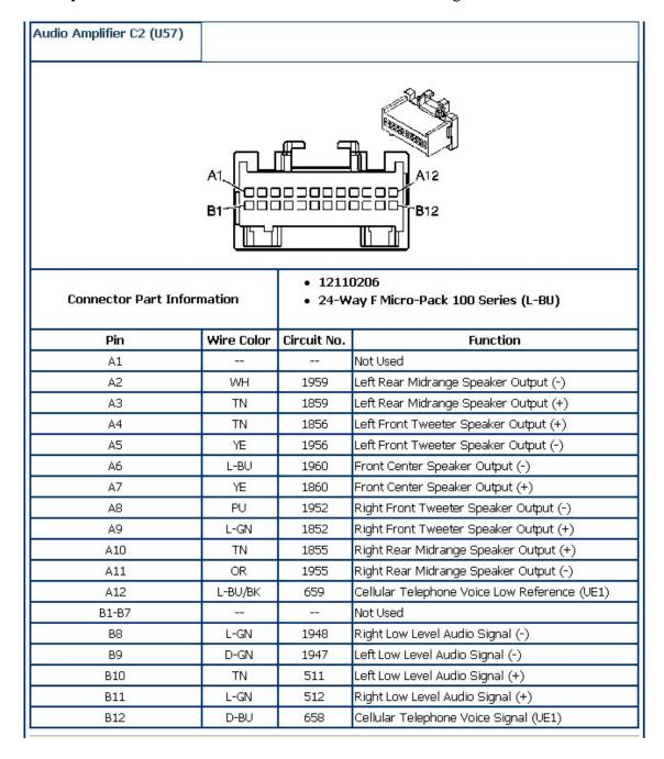
Once you have identified these wires, use a scotch splice to connect the ORANGE wire to B12 and the BLUE wire to A12. This will allow the sound from the Motorola to come through the stereo system.
