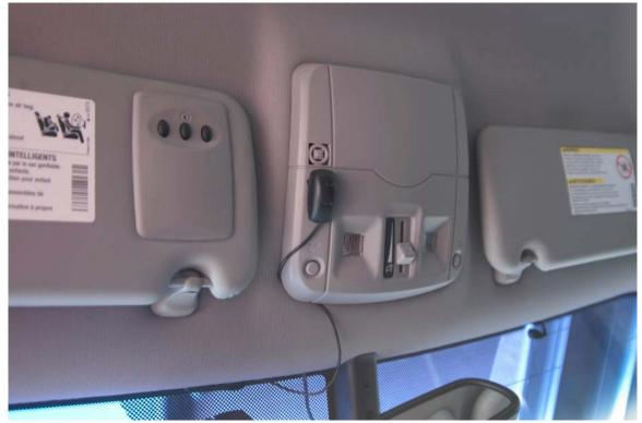
Ignore my laziness in the above photo. I did have the black wire run under the headliner piece at one time, but I removed it since I was adjusting positioning to find the best positioning of the microphone. You can easily run the wire behind the overhead console and then along the front top of the windshield.
