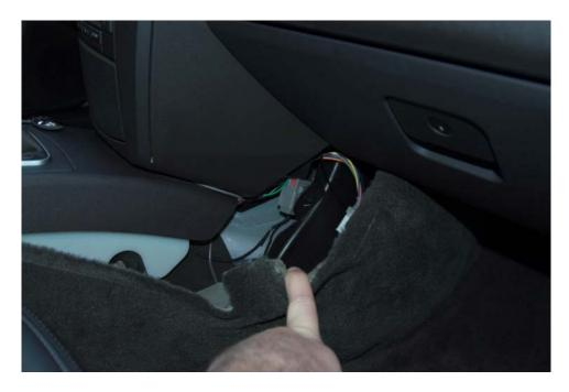
Not place the Blue Motorola interface below the dark plastic piece. Note: I did not mount the Motorola kit. I just placed it there. The weight of the carpet is enough to keep it in place. You can choose to mount it wherever you like if you have a different idea. Next run the end of the harness that connects to the Motorola kit down to the blue box and connect it.
