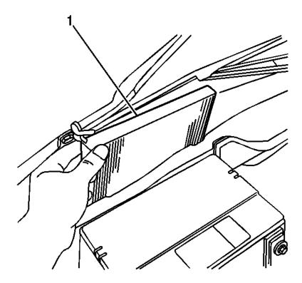
4. Remove the filter (1) from the filter housing.
