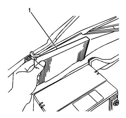
1. Install the filter (1) in to the filter housing.
