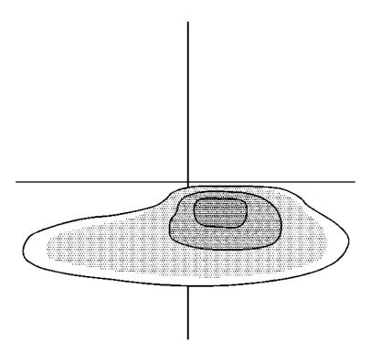
8. Turn on the low beam headlamps and block the light from projecting onto the screen from the passenger side headlamp.
