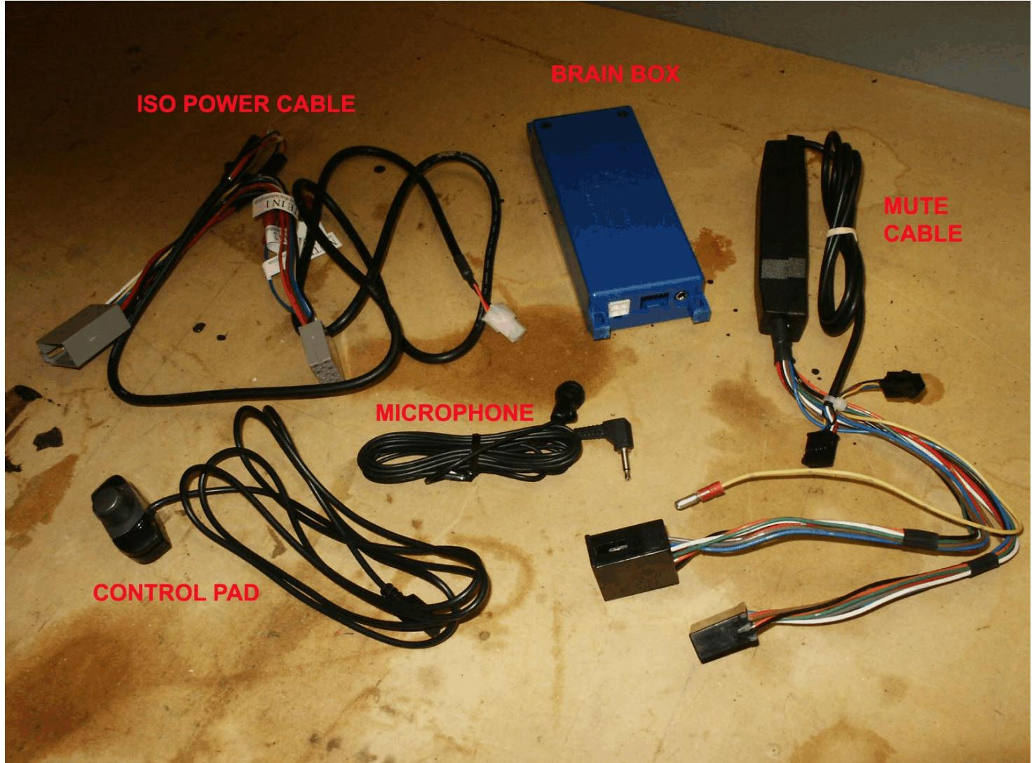
We will only be using half of the ISO power cable, we will cut off the iso connectors just before the fuses. And the control pad will have to be cut, and extension wires spliced in. This is because it is not long enough to reach from the trunk to where I have it mounted. If you mount the brain box under the dash, you will not have to do this.
