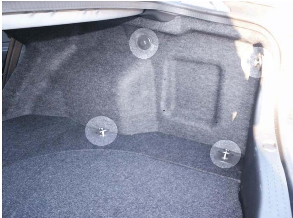
Then remove the spare cover, and the black plastic trim from the lower trunk opening. Just pull up on it, and it will snap off.
