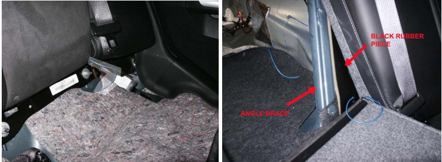
Run the wire along the sidewall of the trunk, tape it in place.
