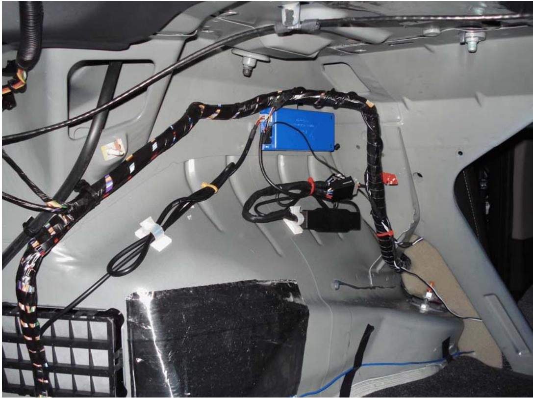
Replace the rear seat. I wedged the speaker between the seat and center hump. It is very securely in place.
