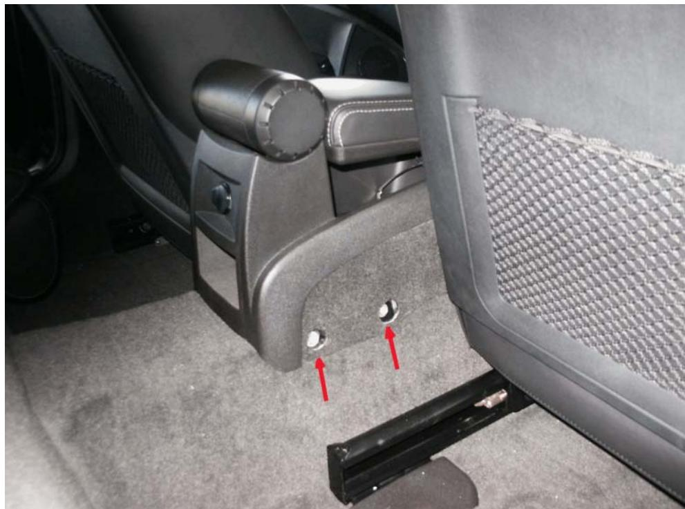
Now lift the console up. You can use a block of wood to support it. Feed a fish tape (if you don't have one, a metal coat hanger will work) as shown below. Get some blue wire, and pull it though.
