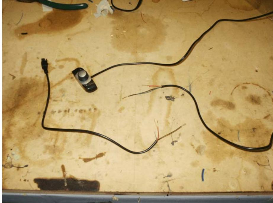
Get some 5 foot section of wires and splice or solder them together (Four wires total). I recommend soldering and do it cleanly, because you will have to tuck this wire into the seams of the headliner. You will have a hard time tucking big clumps of solder or splice connectors.
