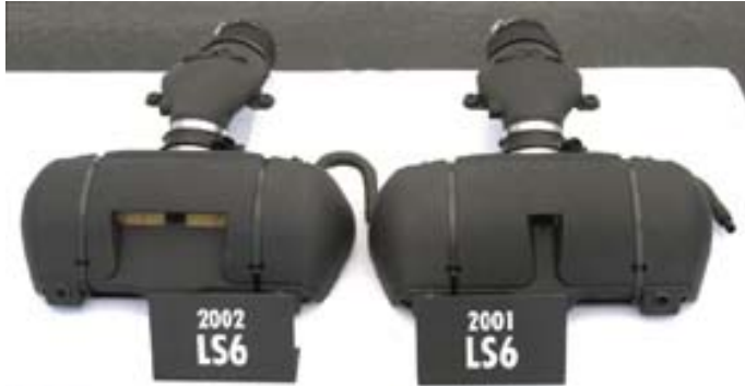
A side-by-side of the '02 and '01 air filter assembly shows their differences. Image: Author [Click Image for Larger View ]
