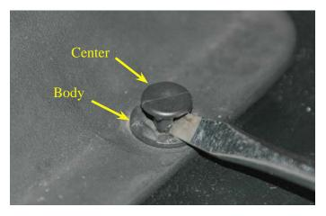
32. Raise the front of the vehicle on jackstands or a lift and remove the lower front splash panel from the bottom of the vehicle. Remove the panel by removing the 13 push rivets in the areas shown.
