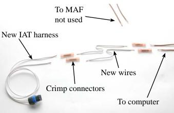
99. Strip about 1/4" of insulation from the ends of all the wires, then crimp the connectors on. Using a heat gun or blow dryer set on "High" shrink the insulation on the crimp connectors so that it contracts around the wires completely. You must shrink the insulation, as crimping the connections alone is not enough to secure them!
