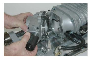
108. Torque the three throttle body bolts to 89 inlbs.
