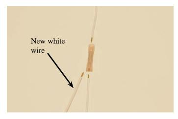
216. After the wires have been connected, cover the length of white wire with the 1/4" split loom supplied.
