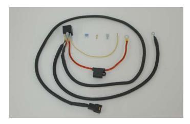
182. Install the intercooler pump wiring harness at the Fuse/Relay center located at the front right corner of the engine compartment. Remove the Fuse/Relay center cover and using the legend printed inside, find the forward fuse location marked "SPARE" as shown.
