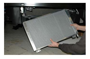
157. Bolt the heat exchanger into place using the supplied Allen bolts and a 4mm Allen socket wrench.
