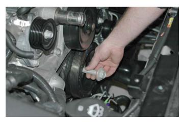
96. Use a torque wrench and 24mm socket to tighten the new balancer bolt to 37 ft-lbs and then rotate it an additional 140 degrees using a torque angle meter. The radiator and hoses will be replaced in a later step.
