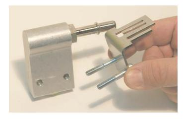
110. Using some of the lubricant supplied, install the O-ring into the recess in the fuel rail. Install the fuel manifold and bracket on the fuel rail, take care not to pinch the O-ring.
