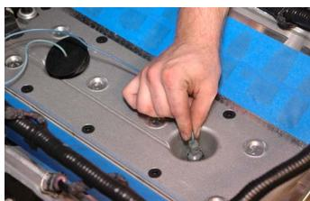
71. Remove the tape from the knock sensor wires so that they can be installed in the grooves in the top of the valley cover. Use some tape to hold the wires in place temporarily, and then use silicone adhesive to retain the wires permanently. Insert the six O-rings supplied in the recesses in the new valley cover.
