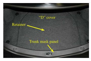
198. Remove the four retainer buttons that secure the trunk mask panel to the rear of the trunk by unscrewing them. There is one button on the floor and one on the wall on each side.
