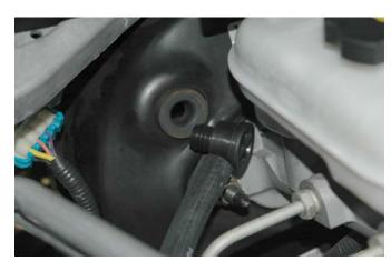
136. On the driver (left) side of the engine connect the brake hose to the large barb on the inlet manifold. Route the brake hose along the side of the engine and behind the supercharger to the brake booster.
