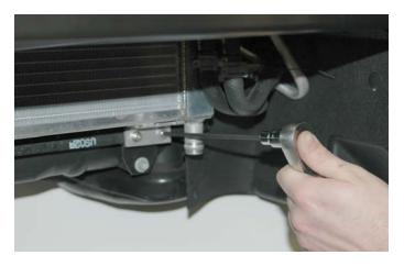
158. Remove the the lower right A/C condensor mounting bolt with a 10mm socket wrench. Install the two reservoir brackets using the A/C mounting bolt and a new supplied bolt in the center attachment point on the radiator tank.
