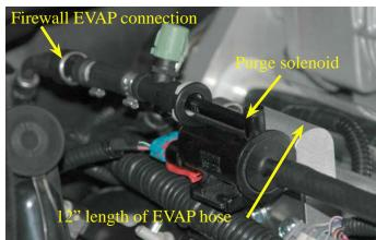
143. Install the fuel line extention into the firewall fuel line connector.
