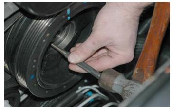
95. Install the new balancer bolt supplied.
