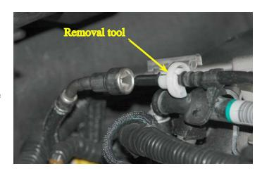
54. Remove the Purge solenoid and EVAP line by pulling the solenoid free from its mounting location on the left side of the intake manifold.
