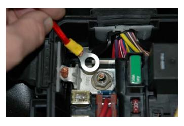
188. Place the relay into the rear corner of the Fuse/Relay center. Using a sharp knife, cut away at the top of the harness boot to allow the ground and pump wire from the relay to pass from the inside to the engine compartment.
