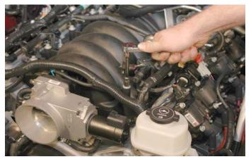
61. Remove the ten intake manifold bolts with a 8mm socket wrench. Note: You may not be able to completely withdrawal all ten bolts from the manifold after unthreading them.
