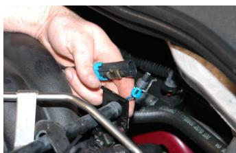
47. Disconnect the Manifold Absolute Pressure (MAP) sensor connector at the rear of the intake manifold.
