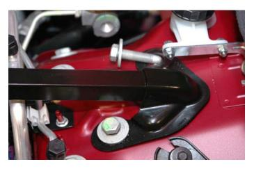
28. Remove the strut tower brace completely, as it cannot be reused with the supercharger. A new strut tower brace is included with this system and will be installed in a later step. Replace the bolts into their original holes temporarily tighten them.
