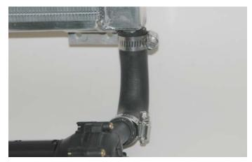
175. Route the large "L" hose through the area created by removing the air box boot. Attach the short leg of the large "L" hose to the outlet barb of the heat exchanger with a #10 clamp.
