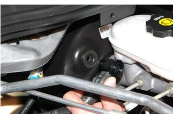
51. Above the drivers (right) side valve cover, disconnect the Evaporative Purge Solenoid (EVAP) electrical connector.
