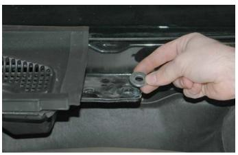
23. Re-install the wiper assembly into place. Note: The mounting bolt will pass through the spacer washer installed in the previous step.
