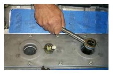
66. Remove the engine valley cover and gasket by removing the ten bolts with a 10mm socket wrench.
