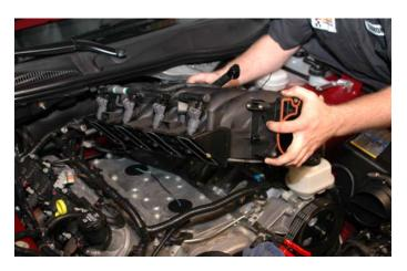
62. Using a shop vacuum cleaner, remove any dirt or debris from the intake port and engine valley cover area.
