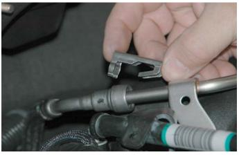
57. Disconnect the fuel pipe from the large quick-release fitting using the supplied removal tool. Snap the tool on the pipe and push it into the quick release fitting to release the pipe.
