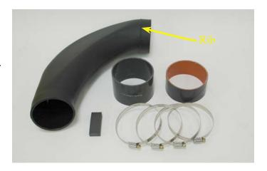
178. Assemble the air tube assembly by sliding the hoses all the way onto the air tube and then place the #60 clamps in position. Note: The shorter of the two hoses will go on the end of the tube with the raised "Rib". Do not tighten the clamps at this time. Peel the paper backing from the rubber pad supplied and attach the pad to the underside of the air tube in the position shown.
