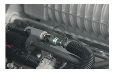
146. Connect the remaining end of the EVAP hose from the purge solenoid to the small barb on the right side of the supercharger inlet manifold.
