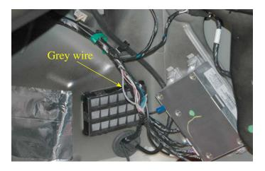
202. Cut the large grey wire and strip the insulation back from the two ends about 1/4".
