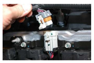
46. Unclip the Engine Knock Sensor (Knock) connector from its location on the back of the intake manifold. Next, disconnect the Knock connector from the wiring harness connector.
