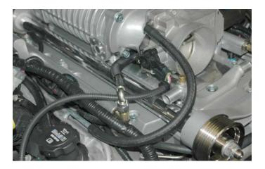
130. At the rear of the driver (left) side valve cover, remove the rubber cap covering the PCV barb.
