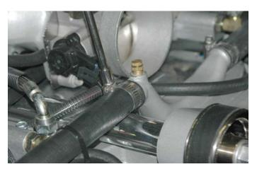
172. Secure the remaining end of the 24" hose to the reservoir inlet barb with a #10 clamp.
