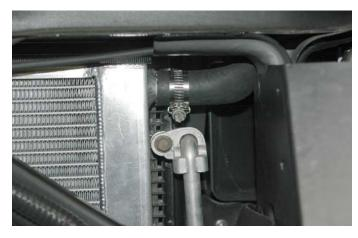
176. Connect the remaing leg of the large"L" hose to the left barb on the intercooler manifold and secure it with a #10 clamp. Tighten all hose clamps securely with a 8mm nutdriver except for the clamp on the right side intercooler manifold barb.
