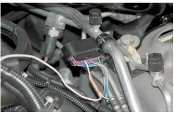
217. Locate at the left rear corner of the supercharger manifold the pressure port and remove the rubber cap. Attach one end of the length of 5/32" hose supplied to the port. The other end of the hose will be routed to the Magnavolt.
