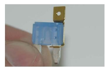
184. Install the new fuse and Fuse-Tap into the "Spare" location.
