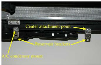
159. Here is the intercooler reservoir tank. Note: The slotted rail on the front surface. Ther are two rails on the back as well.
