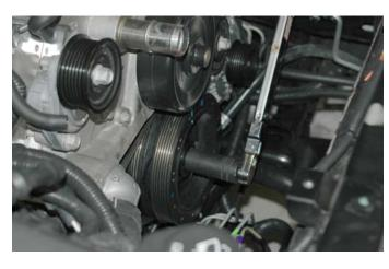
88. Using a drill and the supplied drill bit, drill **Two** holes in the balancer by placing the drill bit in the two holes in the guide. Take your time, as the material will cut slowly. Note: The drill bit has a "shoulder" on it. Continue drilling until the shoulder of the drill bit contacts the drill guide.
