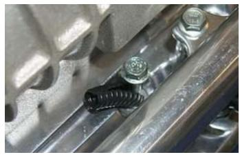
119. Using a torque wrench and 10mm socket torque the ten manifold to cylinder head bolts gradually and evenly to 89 in-lbs.
