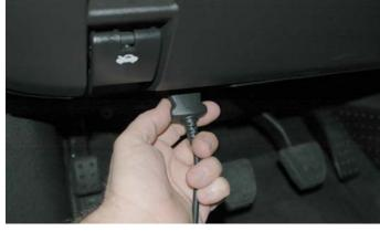
7. Turn the ignition key to the on or run position but do not start the vehicle. To begin programming your vehicle, you must press the YES button. Press the YES button once to start the programming cycle. The programming process takes about five minutes. The handheld unit will inform you that the programming process has completed and to turn the ignition off and disconnect the cable. Only at this time should the ignition be turned off and the cable removed.
