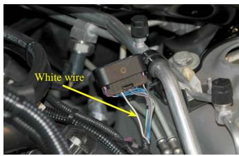
215. Cut the white wire approximately 1-1/2" below the connector. Strip the insulation back 1/4" from both ends of the white wire and connect the ends togather with a end of the new length of white wire supplied. Use a pink crimp/shrink connector to make the connection and be sure to shrink the insulation as crimping the connector alone is not enough to secure the wires.
