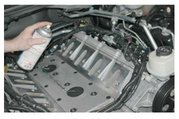
117. With the help of a assistant carefully set the supercharger system in place. Take care not to damage the port gaskets.
