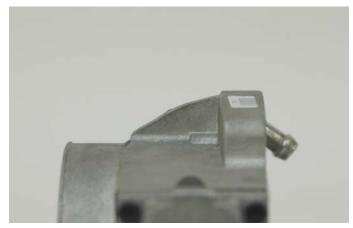
107. Install the throttle body with the new supplied gasket onto the supercharger inlet manifold using the original three bolts and a 10mm socket wrench.
