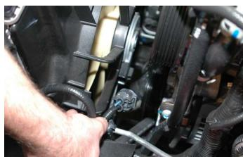
83. Remove the radiator, fan and hoses complete by pulling it straight up and out carefully.
