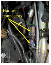
213. Release the connector closest to the front of the vehicle by squeezing the release trigger and pulling it free.
