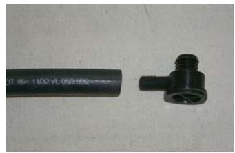
135. Install the new check valve and hose onto the brake vacuum booster.
