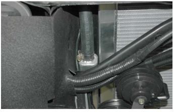
173. Attach the "U" shapped hose to the pump inlet barb and the reservoir outlet barb using the #10 clamps supplied. Tighten the clamps securely with a 8mm nut driver.
