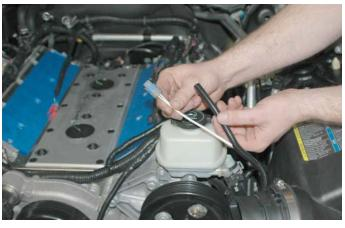
101. Locate the purge solinoid connector and remove the plastic tape. Cut the wires approximately 4" back from the connector.
