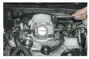
120. At the rear of the supercharger on the passenger side, plug in the MAP and new IAT connections.
