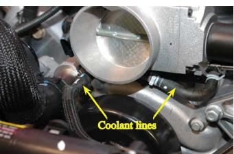
59. Remove the three bolts attaching the throttle body to the intake manifold with a 10mm socket wrench. Set the throttle body and bolts aside for later installation on the supercharger assembly.
