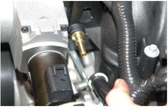
53. Disconnect the Evap pipe from the rear of the purge solenoid. Follow the Evap pipe to the right rear of the engine and unclip it from the fuel rail. Disconnect the Evap pipe from the smaller quick-release fitting using the supplied removal tool. Snap the tool on the pipe and push it into the quick release fitting to release the pipe.
