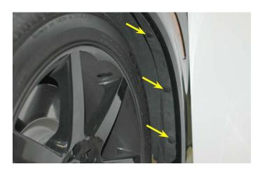
35. Rotate the steering wheel to full lock so you can push the wheel well splash panel out of the way to gain access to the two fascia lock bolts on each side. As you loosen the the nuts on the lock bolts the fascia panel will drop down forming a gap between the fascia and the fender. It is not necessay to remove the lock bolt nuts or the lock bolts themselves.
