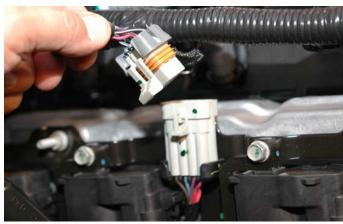
123. Install the connecors on all eight fuel injectors.
