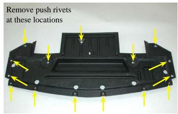
33. Remove the eight push rivets that secure the top edge of the front fascia as shown.
