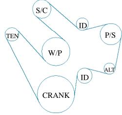
152. Using a long 15mm wrench to compress the tensioner, install the new belt using the diagram above.
