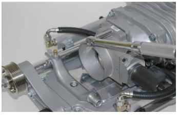
109. Assemble the Evap solenoid bracket and bolts onto the fuel manifold.
