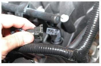
45. Disconnect the two ignition coil pack connectors.
