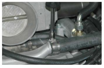
177. Here is the air tube assembly components. Note: The two different lengths of hose and the raised "Rib" around one end of the tube. This end of the air tube will go towards the throttle body.
