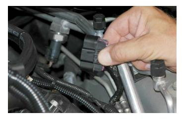
214. Remove the insulating tape below the connector and locate the solid **WHITE** wire. This is the Engine Speed Signal (RPM) wire.
