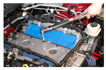
70. Reinstall the knock sensors and torque them to 15 ft-lb. Re-attach the electrical connectors by pushing the connector down firmly until a "click" is heard. Before re-installing the covers, apply a bead of silicone adhesive to the sides of each cover then push the covers back into place.
