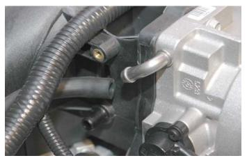
49. Disconnect the engine valley cover vent hose from the nipple in the intake manifold.
