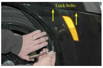
36. The lock bolts are located before and after the marker lamp, where the fascia panel meets the fender as shown in this photo from the inside of the fascia.
