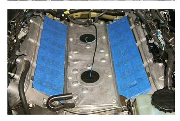
64. On the engine valley cover, remove the two black rubber Knock Sensor covers by gently prying them up using a small straight blade screwdriver. Disconnect the electrical connectors by squeezing the sides of the connectors with a pair of long jaw or needle nose pliers and pulling them up.
