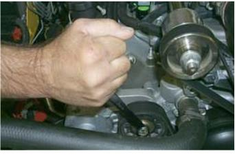
153. Re-install the radiator into the vehicle. Reinstall the radiator hoses, fan electrical connections and A/C line support tab. The radiator mask will be installed in a later step.
