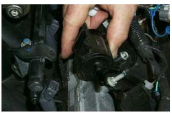
55. On the left side of the intake manifold, locate the fuel pressure test port at the front of the fuel rail and remove the cap. CAUTION! The fuel in the system is under pressure! Relieve the pressure in the system by depressing the check valve with a screwdriver and collecting the fuel with a shop towel.
