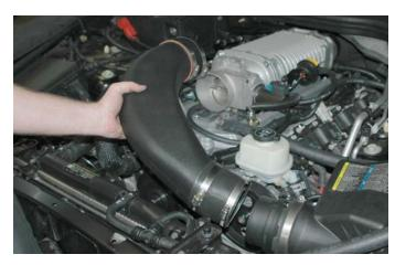
180. Slide the hose and clamp onto the throttle body and then tighten all the hose clamps securely with a 1/4" nut driver.
