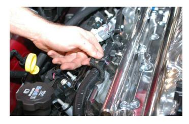
124. Install the TPS extention harness onto the harness connector.
