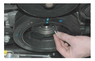
94. Use a small hammer and a drift to tap the dowel pins in as far as they will go into the balancer.
