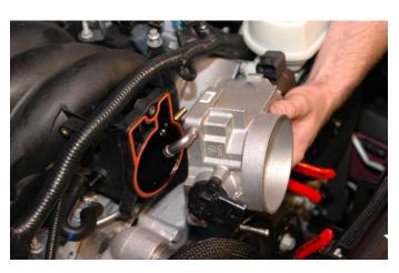
60. Remove the three bolts attaching the throttle body to the intake manifold with a 10mm socket wrench. Set the throttle body and bolts aside for later installation on the supercharger.
