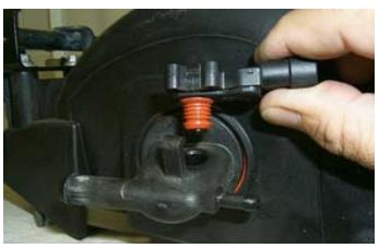
113. Apply a small amout of the grease supplied to the MAP sensor seal and install the sensor in its new location at the right rear of the supercharger manifold.
