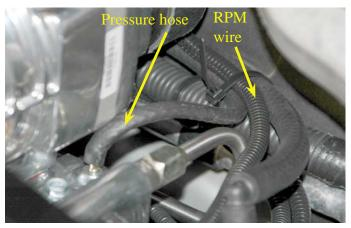
219. Trim the pressure hose to length and using the hose connector supplied, connect the hose to the Magnavolt unit.
