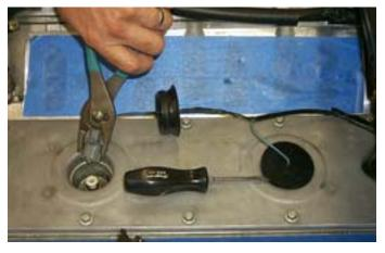
65. Remove the Knock sensors by using a ratchet and a deep 22mm socket.
