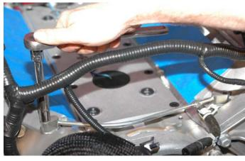
73. Remove the coolant vent pipe. Ensure that the O-ring gaskets under the vent pipe blocks do not stick to the cylinder heads. If so, remove them as new gaskets are supplied.
