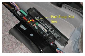
4. Remove the stock "**Fuel Pump Mtr**" fuse and replace it with the 30 amp fuse supplied. Replace the fuse center cover.
