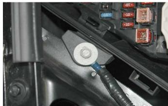
187. Connect the Red positive (+) wire with the ring terminal to the main power connection on the Fuse/Relay Center. Remove the nut with a 13mm wrench and place the ring terminal on the stud. Reinstall the nut and tighten it securely.
