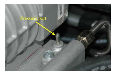
218. Secure the hose and RPM wire to the harness where it pases behind the supercharger with the tie straps supplied. Route the hose and the RPM wire around the back of the supercharger assembley along the fire wall and battery to the Magnavolt unit.
