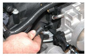
50. Disconnect the vacuum brake booster valve from its mounting grommet on the booster.
