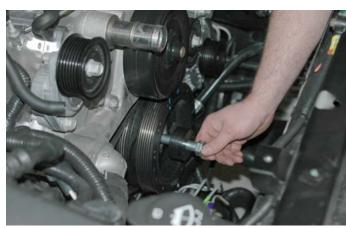
87. Torque the guide bolt to 60 ft-lbs with a torque wrench and 24mm socket.
