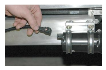
190. Re-install the front fascia by first re-connection the four electrical connectors on the inside of the fascia. Note: The heads of the lock bolts in the top edge of the fascia, these must stand proud in order to engauge the "keyhole" slots in the bottom edge of the fenders.
