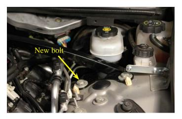
210. Torgue the forward strut tower bolt on the passenger side first to 83 ft-lbs. using a 18mm socket and torque wrench. Next, install the new strut tower brace on the passenger side by first passing the two mounting bolts through the Magnavolt mounting bracket. Torque the remaining strut tower bolts on each side (six in total) to 83 ft-lbs.
