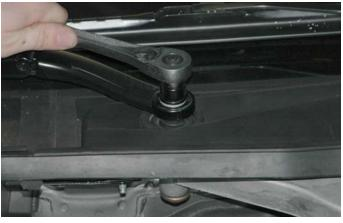
13. Note: The position of the wiper arms on the windshield and then pull up firmly to remove the wiper arms.
