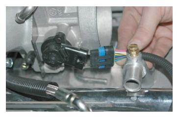
126. Install the ETC connector onto the throttle body.
