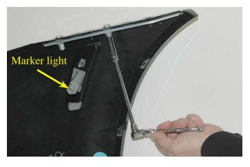
37. After loosening the lock bolts, pull forward on the fascia panel. The lock bolts will slide forward in their "keyhole" shaped holes and allow the fascia to detach from the vehicle.
