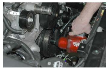
86. Install the drill guide and bolt into the stock location. Note: The smaller diameter end of the guide goes towards the balancer.
