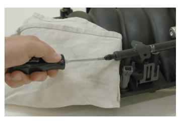
56. Remove the retaining clip from the fuel line quick-release connection.
