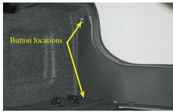
199. Remove the trunk mask panel from the trunk compartment.
