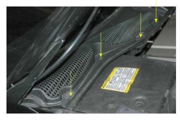
16. In the corner of the left (driver) side wiper apron, remove the bolt that secures it with a 10mm socket wrench.
