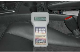
8. \*DO NOT DISTURB THE CABLE OR TURN THE IGNITION OFF DURING THIS TIME! IF THE PROGRAMMING IS DISRUPTED YOUR COMPUTER WILL NOT START OR RUN YOUR VEHICLE! If you should get the message "ERROR NO VIN STORED OR THIS MODEL YEAR NOT SUPPORTED" on the Microtunner display, remove the cable and Microtunner from the OBD II port and take your vehicle back to your Cadillac dealer and ask to have your PCM program updated to the current program.
