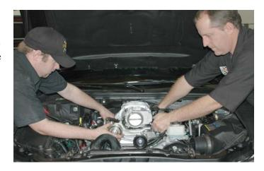
118. Remove the split-looms that support some of the manifold to cylinder head bolts. Start all ten bolts by hand to ensure proper alignment of the manifold.
