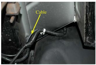
207. Route the cable forward along the brake and fuel lines to the firewall on the passenger side strut tower area of the engine compartment. Take care to keep the cable away from any rotating or hot exhaust parts. Secure the cable with the cable tie straps supplied.
