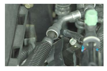
144. Connect the remaining end of the fuel line extention to the fuel manifold connector
