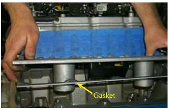
69. Install the new valley cover and ten flathead bolts supplied with a 5mm Allen socket. Torque the bolts to 18ft-lb.
