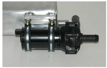
163. Install the two remaining round head bolts into the rails on the back of the reservoir.
