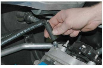
133. Install the plain end of the 43"PCV outlet hose on the passenger (right) side of the engine.
