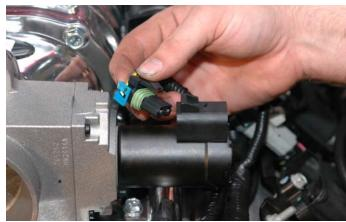
127. Install the purge solenoid onto the new bracket and then install the EVAP electrical connector.
