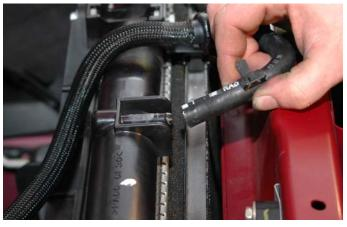
81. On the left side of the engine, remove the A/C pipe support tab from the fan shroud with a right angle cross-head screwdriver.
