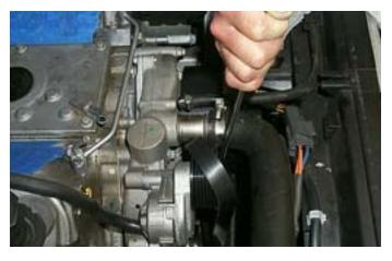
68. The gasket will be reused, the original valley cover will not. Inspect the gasket for any damage and then re-install. Note: It will only fit correctly in one position.
