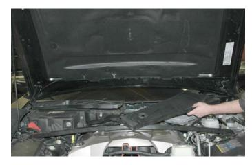
18. Located on the bottom of the wiper assembly is the wiper motor electrical connector. Disconnect the connector from the motor.
