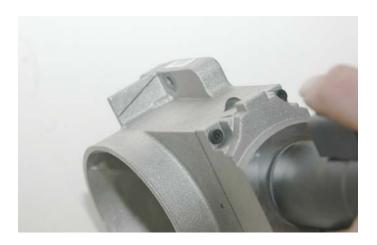
106. Using a small saw or grinder carefully remove the material above the line until the throttle body looks like this.
