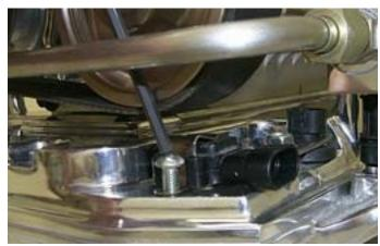
115. Install the new intake manifold gaskets supplied onto the recesses in the manifold face. Ensure that the gaskets are fully seated in the manifold face.
