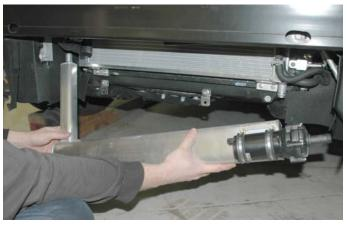
165. Secure the reservoir and pump assembly to the bracket uisng the supplied nuts. Tighten the nuts securely with a 12mm wrench.
