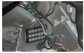
203. Using the large grey cable supplied strip back the outer grey covering and strip 1/4" of the insulation off the ends of the black and white wires. Install the cable using blue crimp/shrink connectors supplied. Connect the large **BLACK wire to the Upper grey wire.** Connect the remaining large **WHITE wire to the lower grey wire** that runs to the fuel pump.
