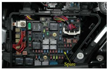
183. Place one leg of the supplied 15amp fuse through the Fuse-Tap as shown.
