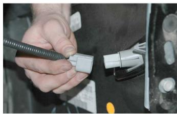
39. On both sides of the fascia disconnect the turn signal/driving light electrical connection. Remove the fascia carefully from the vehicle and set it aside.
