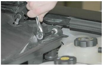
17. Pull the right wiper apron forward at the center, then remove the left apron completely.
