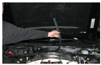
15. Remove the four 7mm bolts that secure the wiper apron on the right (passenger) side.
