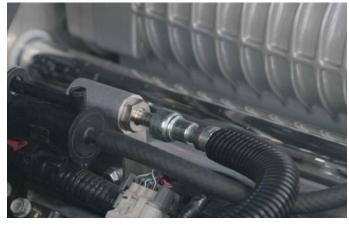
145. Re-install the fuel line retaining clip.
