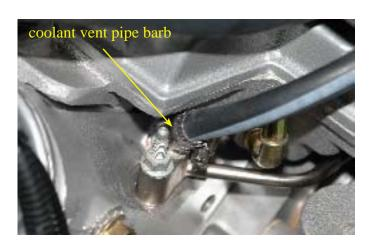
150. Connect the remaining end of the 20" coolant hose to the left side throttle body barb using a #4 clamp supplied.
