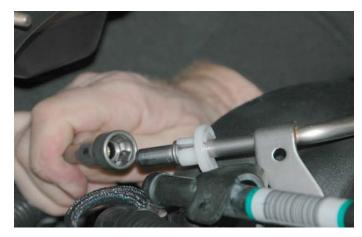
58. Remove the two coolant lines attached to the bottom of the throttle body.
