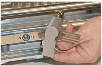
111. Torque the fuel manifold bolts to 106 in-lbs with a torque wrench and 10mm socket.
